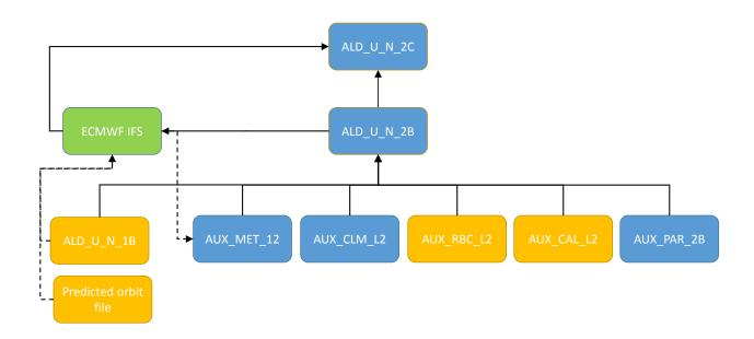
Figure 1: Relationship of Input/Output Files for the Aeolus Level-2B Processor
