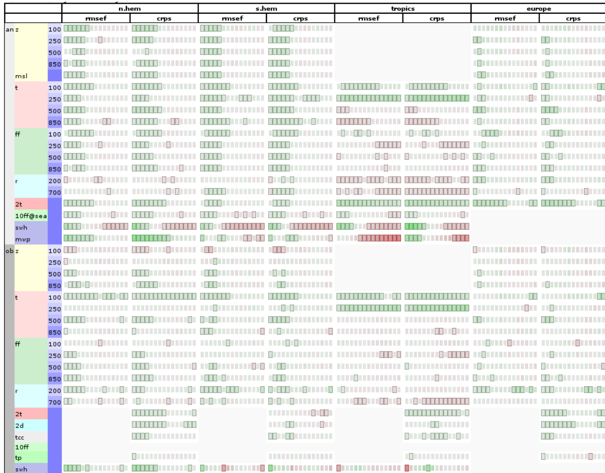
Figure 6: Combined summer/winter TCo399 ensemble scorecard for different meteorological fields. The 46R1 version including the merged model and data assimilation changes is compared with a baseline version which is equivalent (completely neutral) to 45R1. Green colours indicate improvement against the baseline version while red indicate deterioration.
