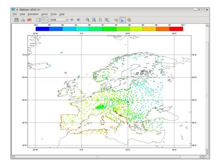
We used the **Symbol Table Mode** in our icon and set it to 'Advanced' which enabled us to automatically define intervals with a separate maker type, colour and size. These settings work in a similar way as in the *Contouring* icon.
