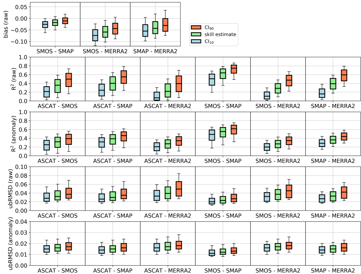
Figure A.9: Spatial summary statistics of biases [ m^3m^{-3} ], ubRMSDs [ m^3m^{-3} ], and coefficients of determination [-] and their 10% and 90% confidence limits, respectively, for raw soil moisture estimates and soil moisture anomalies of ASCAT, SMOS, SMAP and MERRA-2. Boxes represent the (spatial) median and inter-quartile-range and whiskers represent the 5 and 95 percentiles.
