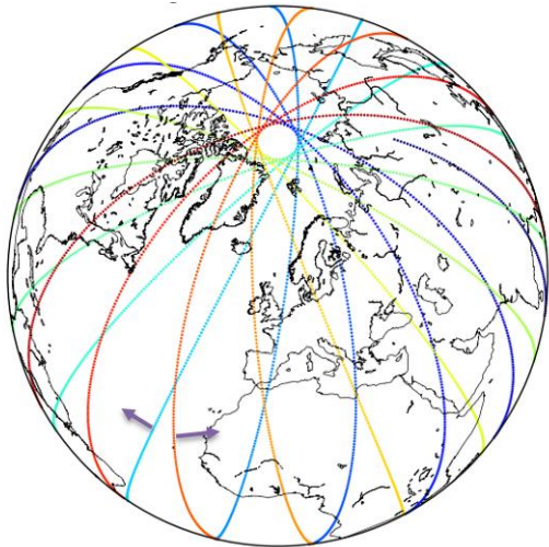
Figure 2. An example of Aeolus near surface geolocations in one day. The line-of-sight pointing of ALADIN is indicated by the purple arrows for an ascending (Eastwards) and descending (Westwards) orbit. The higher spatial sampling near the north pole is evident.
