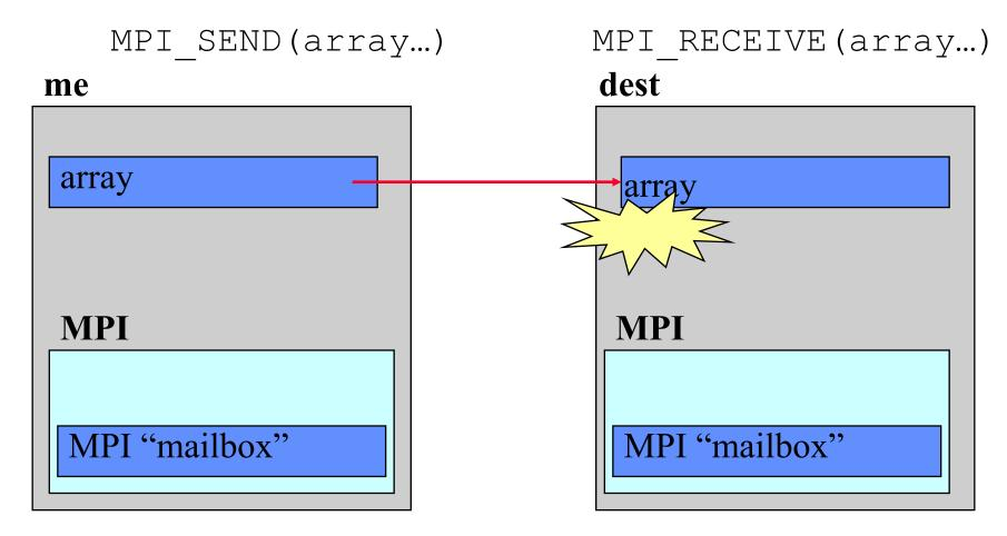
MPI\_SEND completes when "array" is copied into "array" on the receiving task
