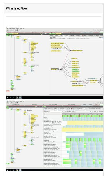
**ecFlow** is a client/server workflow package that enables users to run a large number of programs (with dependencies on each other and on time) in a controlled environment. It provides reasonable tolerance for hardware and software failures, combined with restart capabilities. It is used at ECMWF to run all our operational suites across a range of platforms.
