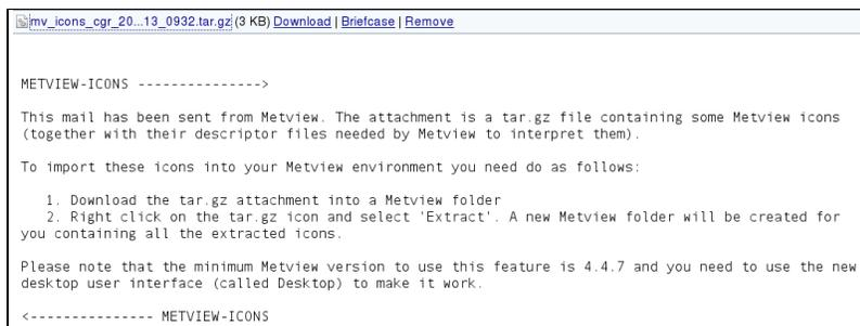
The automatically generated part of the message contains clear instructions on how to import the icons in the tar.gz attachment into the local Metview environment.
